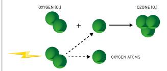
To produce ozone you need energy and oxygen. Energy comes from electricity, while the oxygen is generated from the ambient air or from an oxygen generator.
