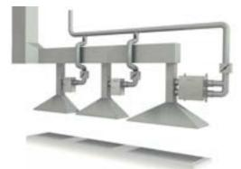
A stainless steel (SS316L) ventilation duct connects the grease duct and the FTX ozone generator.
