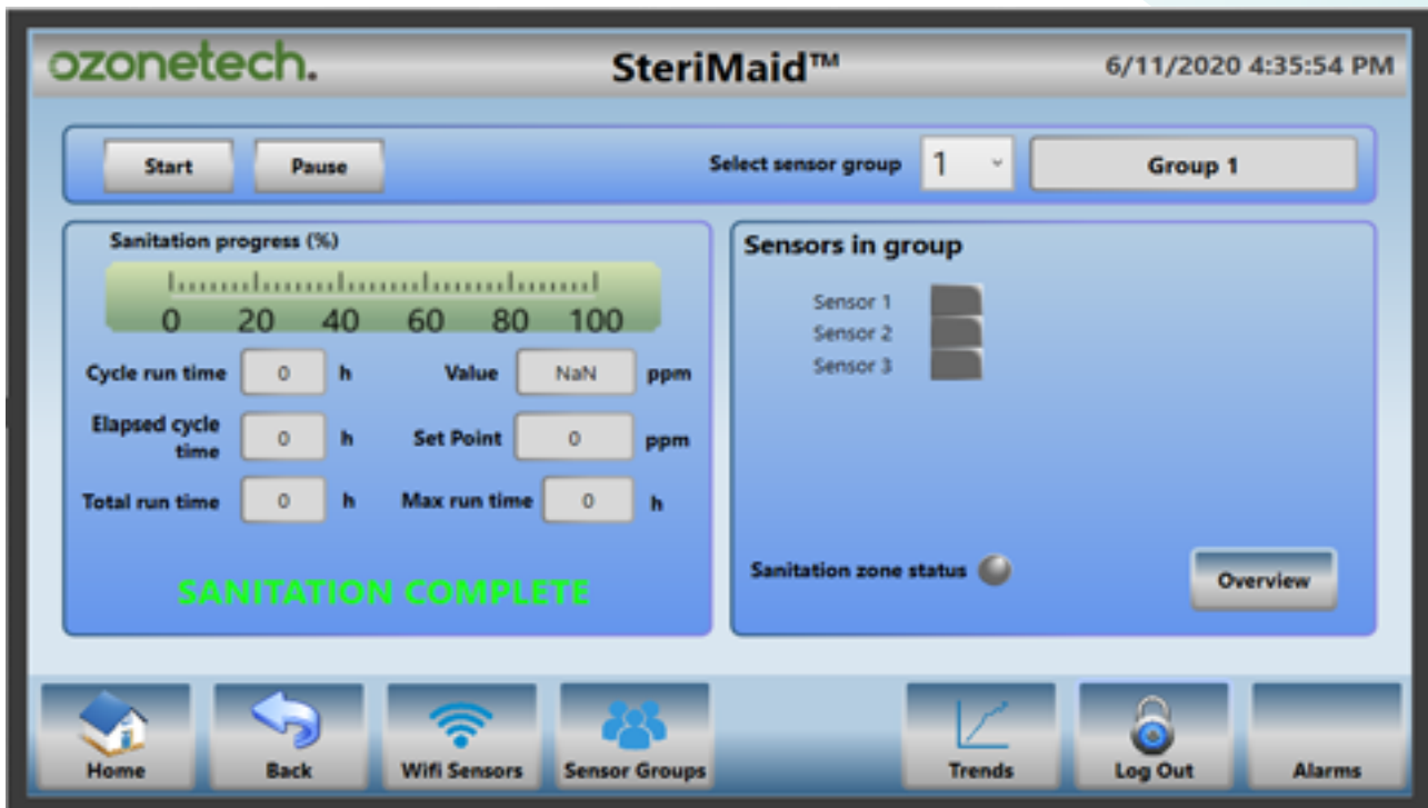
The home screen of the SteriMaid™ with wireless ozone sensor communication.
