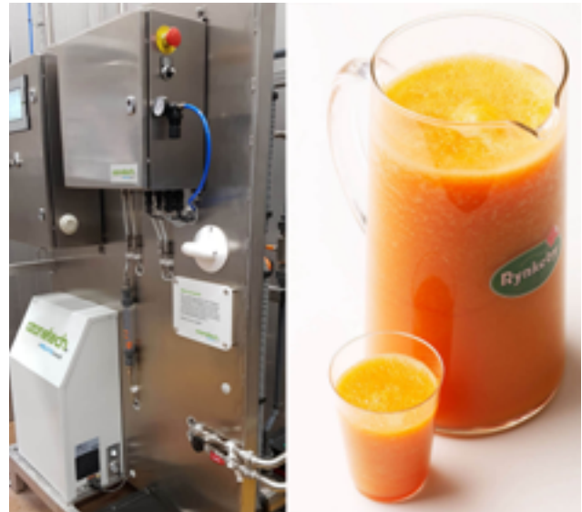
The Ozonetech RENA Vivo A3 system ozonates the fruit rinse tank to programmable set-points.
